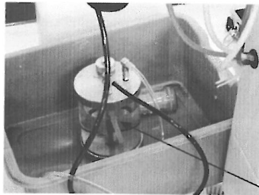
Fig. 1-B. Inflow of acidic electrolyzed water into the piping box.
